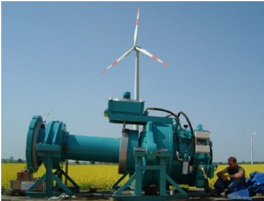
The New Gearbox from Lohmann&Stolterfoht waiting to be installed
